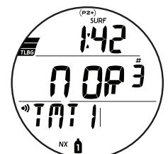
Fig. 6 - SURF MAIN (TMT low battery alarm)
